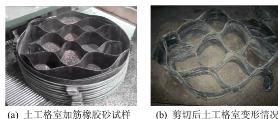
图12 加筋橡胶砂试样 Fig.12 Specimen of geo-cell reinforced rubber sand mixture for testing
